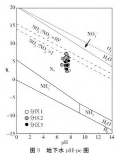
Fig. 9 Groundwater pH-pe diagram
